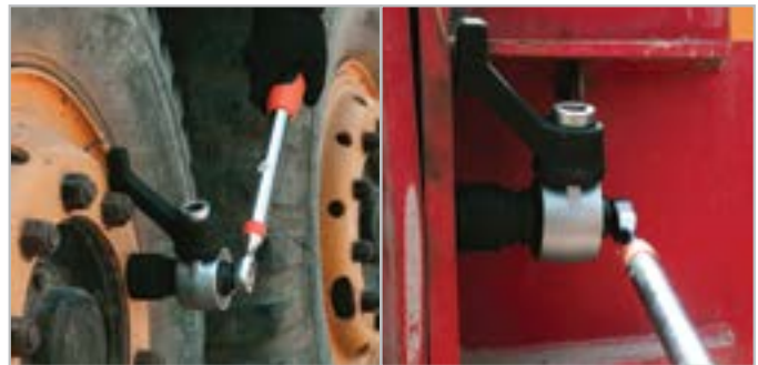
Foot reaction bar for obstacles at short distance
