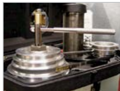
Draw Bar Hammer - being used to loosen a nut on a pulley drive
