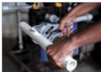
Cuts upto 1-21/32" (42mm) dia pipes
