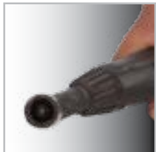
Welding Gun Nozzle filled with weld splatter
