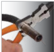
Nozzle removal & installation
