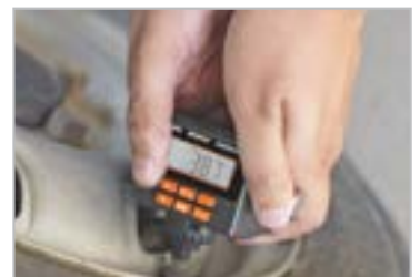
MODE 2 Use as Tyre pressure gauge
