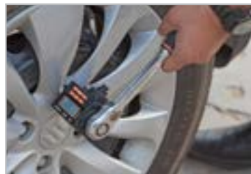
MODE 1 Use as digital torque adaptor
