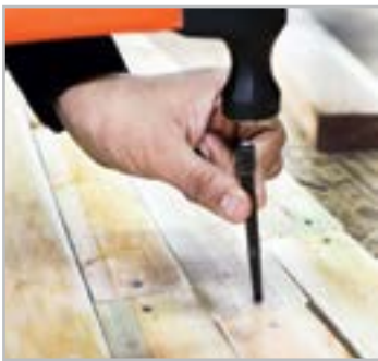
The working end is cupped to follow the nail head without sliding off
