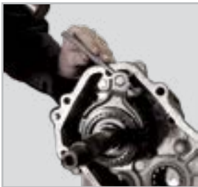
Pin Punches are used for driving out and removing already loosened pins & keys after initial movement by a solid or starting punch
