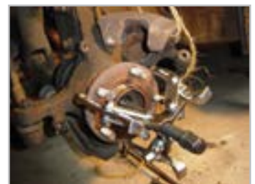
3 Jaw Puller used for removing tyre hub
